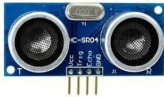
HC-St04 ultrasonic sensor
